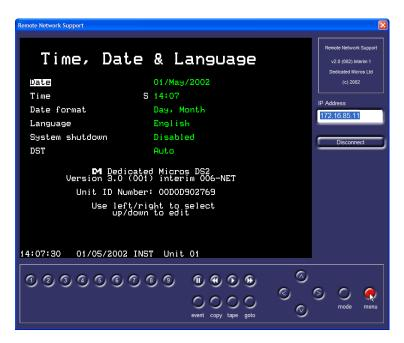
The menus you see are identical to the menus that are configured at the unit locally, any changes you make will be seen on the digital recorders main monitor. Click on the cursor keys to move the highlighted cursor around the screen, and edit the options. Click on the 'menu' button to move to the next menu page. Once you have finished configuring the digital recorder, click on 'Disconnect'.
